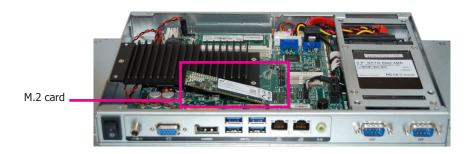
4. Push down on the other end of the M.2 card and secure the card on the mainboard with the provided mounting screw.
