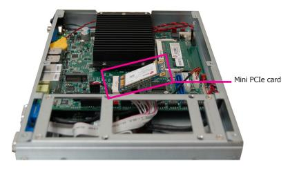
2. Push the Mini PCIe card down and use the provided mounting screws to secure the card on the system board. Route the antenna cables underneath the SATA bracket to the reach the antenna holes on the side panel.
