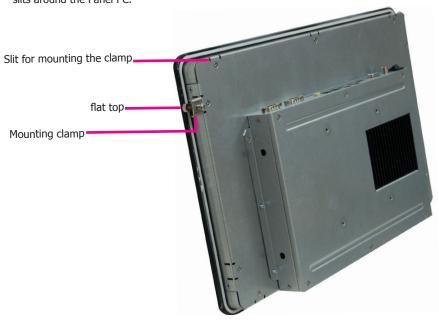
The first and second clamps must be positioned and secured diagonally prior to mounting the rest of the clamps. Tighten the clamp's screw using an electric screwdriver by pressing the white plastic cap onto the back of the panel. The illustration below shows that all clamps are properly mounted.
